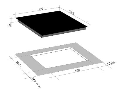
\*Note: The safety distance between the hotplate and the cupboard above the hotplate should be at least 600mm
