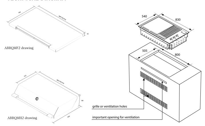
\*Please note that installation specifiations and requirements differ depending on if the unit is installed indoors or outdoors. Please refer to the relevant installation manual for full details
