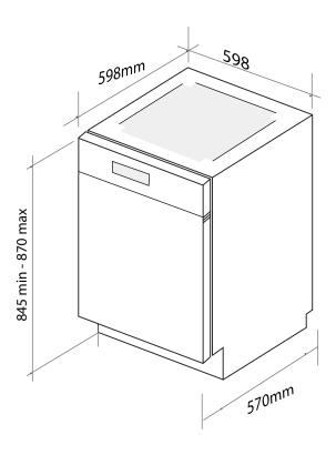
Note: For built-in installation, please remove the lid of the appliances. Refer to the installation manual
